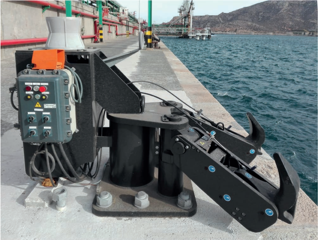
QRH showing local control panel. GER mostrando el panel de control local.
