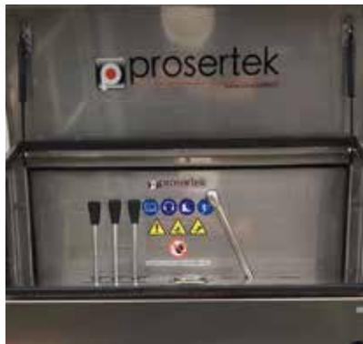
**The main actuators and operative ranges are hydraulic** taking advantage of the fact that with low energy and small elements, huge strength and power can be produced and transmitted. The hydraulic control device and valves provide simplicity and robustness that ensure operability.
