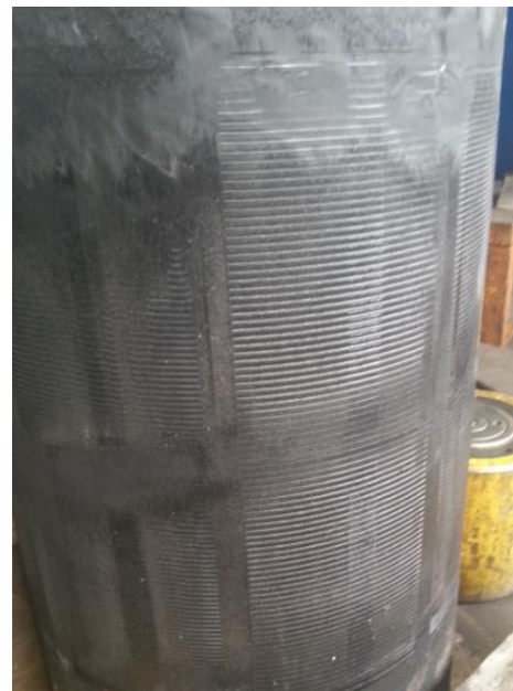
Surface Condition after 100 t Load
