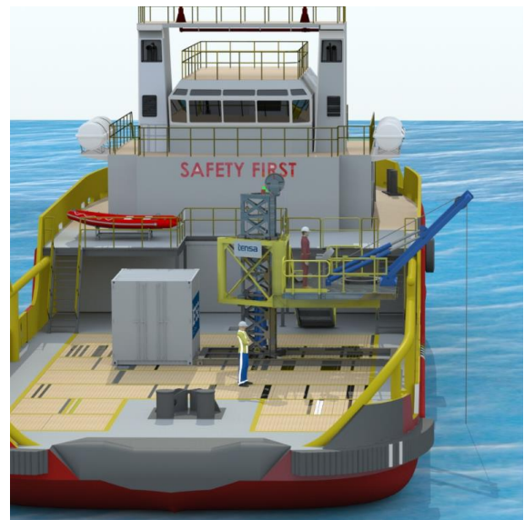
Supporting A frame and winch
