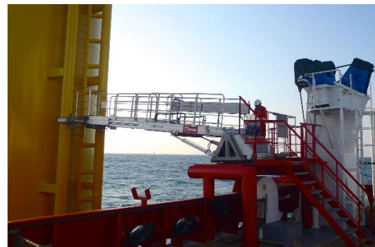
Operating in gripper mode using passive heave compensation to support the gangway weight.
