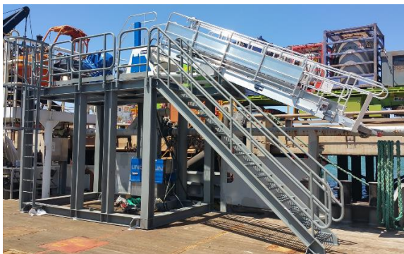
Gangway and support structure can be installed very quickly in a single lift.
